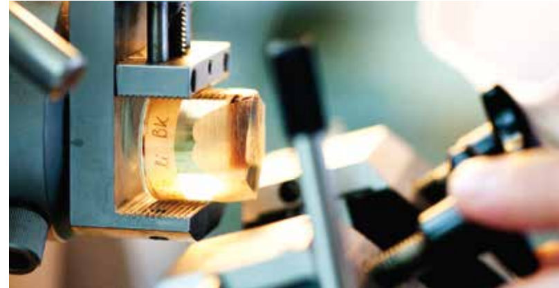
A bone sample is embedded in a block of plexiglas and cut into slices thousandths of a millimeter thick by a microtome which is part of our core facilities
